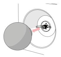
Unscrew the 2 x brass dome headed screws to release the wall fixing plate from the back of the shade.
